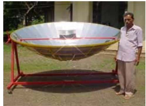
The parabolic solar cooker is more efficient than the conventional solar cookers
